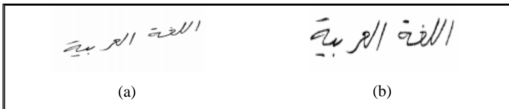
Figure (2.3) skew correction of word "اللغة العربية" (a) Original image (b) the result of skew correction
