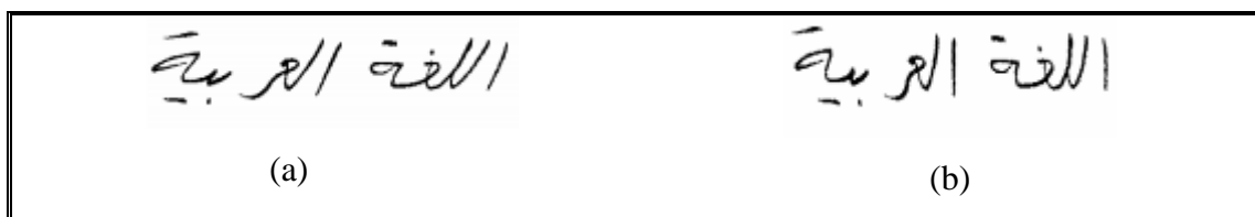
Figure (2.4) slant correction of word "اللغة العربية" (a) Original image (b) the image after apply slant correction
