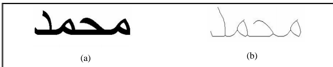
Figure (2.5) thinning of word "محمد" (a) Original image (b) the result of thinning process
